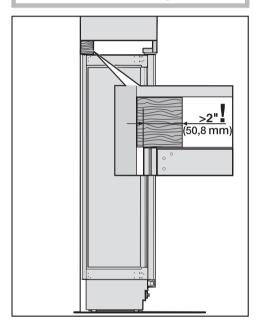
■ Cut a wooden beam (cross section min. 3" x 4" [75 mm x 100 mm] to the required length).
